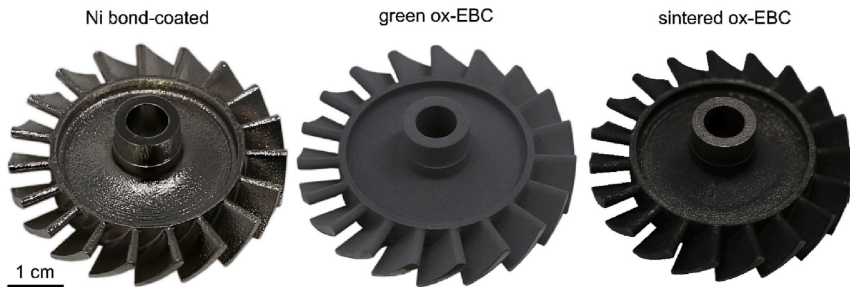
Fig. 2. Macrograph of an IN718 blisk with a Ni bond coat, a green ox-EBC, and a sintered ox-EBC. (For interpretation of the references to colour in this figure legend, the reader is referred to the web version of this article.)
